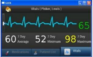
GUI designs (as shown in the Figure). With GUIX Studio, the designer can select, drag-and-drop, and resize images, backgrounds, widgets, and other elements of a powerful GUI without having to write a single line of code. GUIX Studio generates the code necessary to implement the exact GUI design constructed on the PC. The generated code can be dropped into the application and
